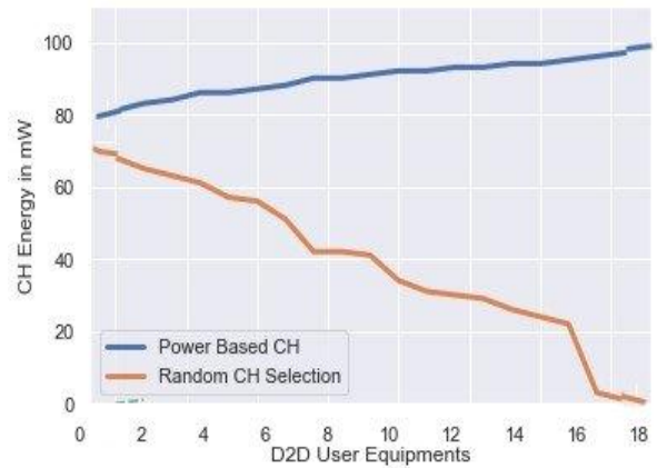
Figure 4.3 Residual Energy-Based Cluster Head
