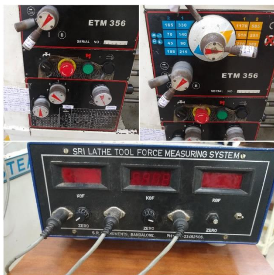
Figure 2: Lathe Machine And Machine-Tool Dynamometer
