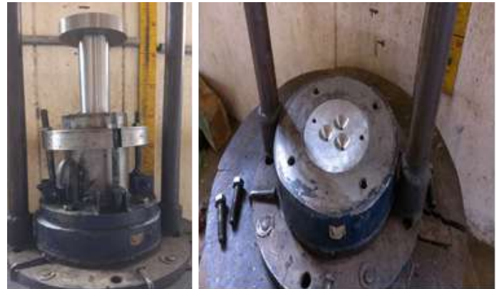
Fig-2 Experimental Setup & Multi cavity Die
