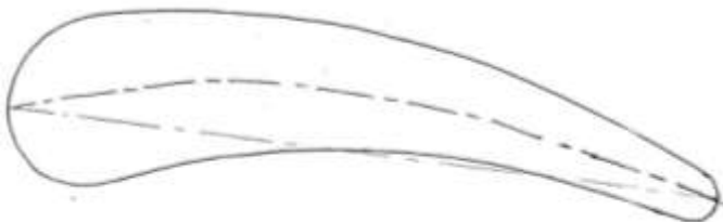
Fig. 6. The Cambered – Cambered Aerofoil Drawn in Full – Size Dimensions
