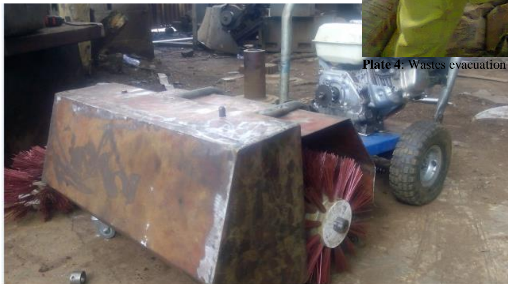
Plate 2: The fabricated portable sweeping machine
