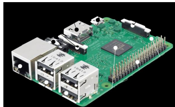
Fig. 1. Raspberry Pi board Raspberry Pi is having 5V, 3A, full power delivery to USB devices. It is having a CPU of 1.5GHz, 64/32-bit quad-
