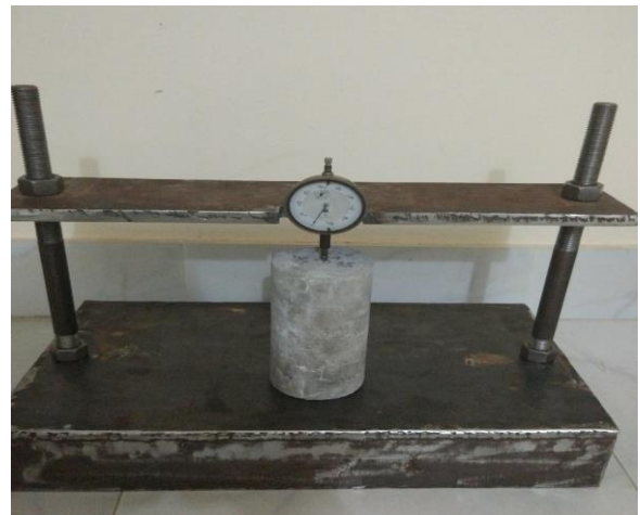
Fig. 1. Length comparator with tested material.
