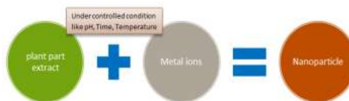
Figure 3: One stage synthesis of nanoparticles
