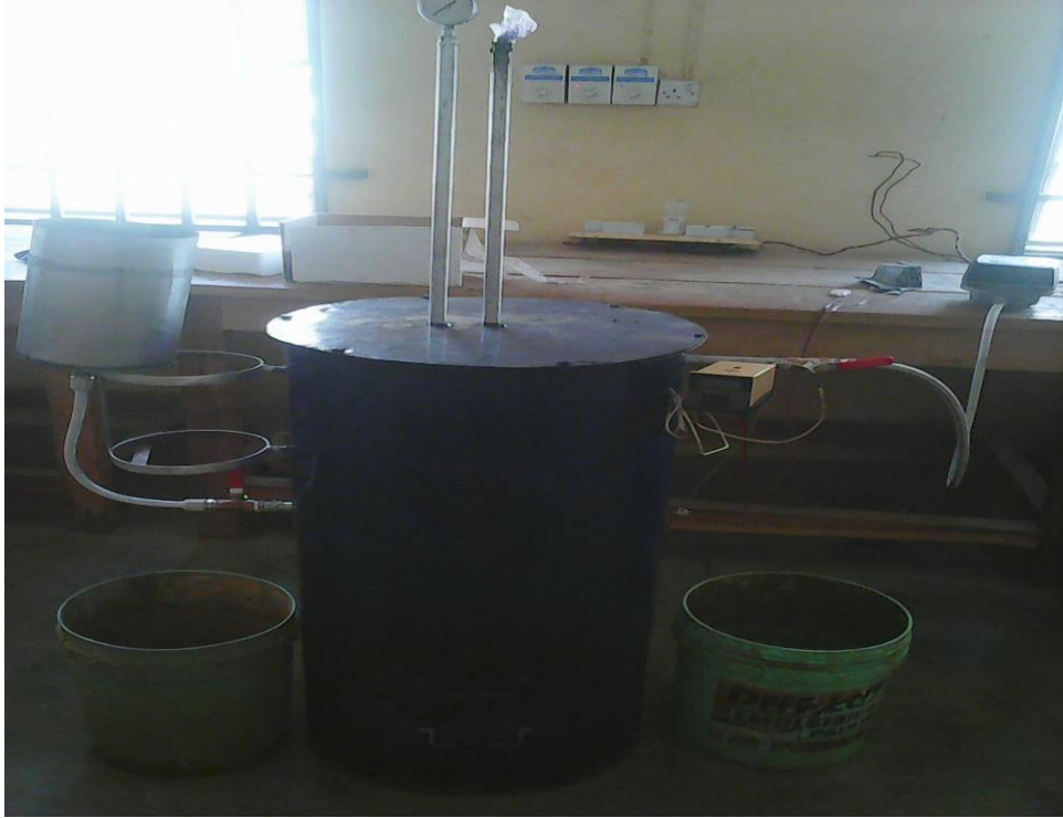
Plate 2: Steam Boiler which was the source of the steam being injected into the sandbox
