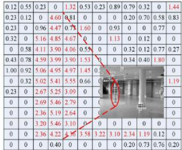
Fig 3 Block-Based Entropy Value in a Video Frame
