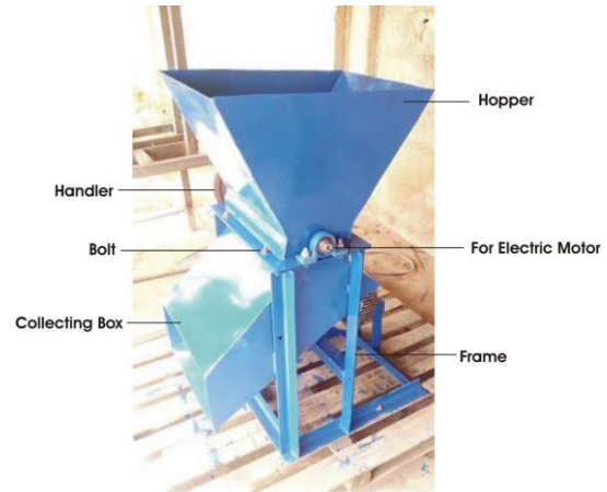
Figure 1.1: Dual Power Operated Cassava Grating Machine
