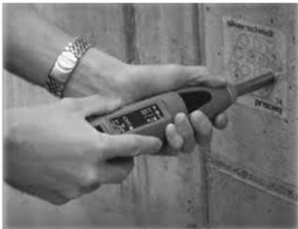
Figure 1: NDT of concrete by Schmidt Rebound Hammer
