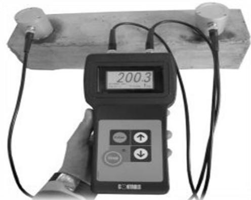
Figure 3: Ultrasonic pulse velocity test apparatus
