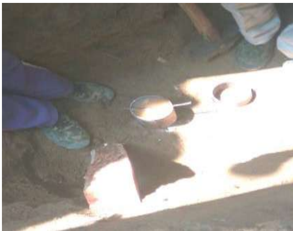
Fig. 3. Measurement of In-situ permeability
