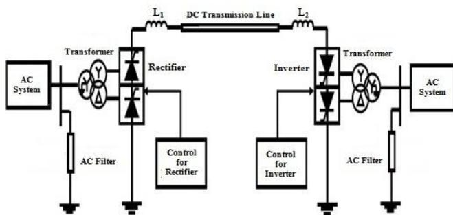
Fig 1. The monopolar HVDC transmission system model
