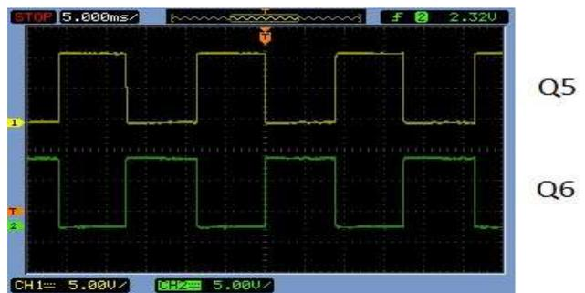
Fig. 12. Gate pulses of Switches Q5 and Q6
