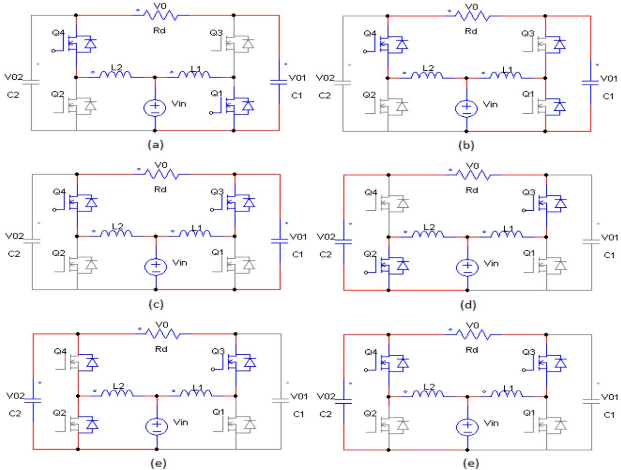
Fig. 4. Equivalent circuits of switching modes. (a) [ $t_0, t_1$ ], (b) [ $t_1, t_2$ ] or [ $t_3, t_4$ ], (c) [ $t_2, t_3$ ], (d) [ $t_6, t_7$ ], (e) [ $t_7, t_8$ ] or [ $t_9, t_{10}$ ] and [ $t_{10}, t_{11}$ ]
