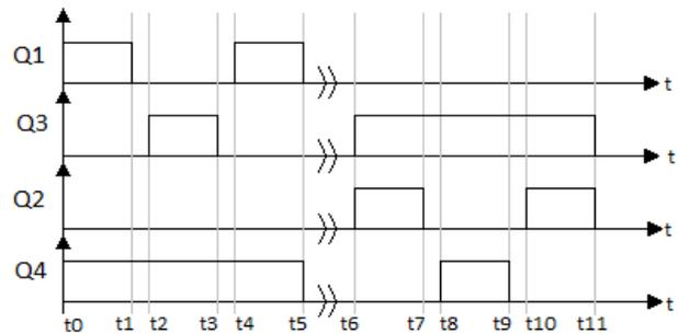
Fig. 3. Control strategy under half cycle modulation.
