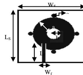
(C) 2<sup>ND</sup> ITERATION STAGE OF CIRCULAR FRACTAL ANTENNA
