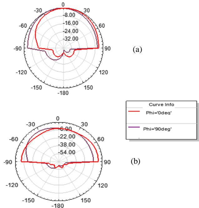
Fig. 5. Simulated radiation pattern of Ist iteration at (a) 3.10GHz (b) 7.76 GHz
