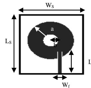
(B) 1<sup>ST</sup> ITERATION STAGE OF CIRCULAR FRACTAL ANTENNA
