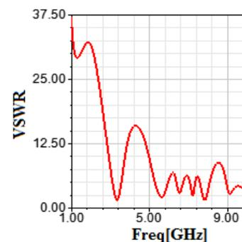
Figure 3. Simulated VSWR of (a) 0th iteration stage,
