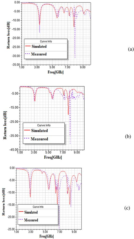
Fig. 9. Simulated and measured return loss vs. frequency plot of (a) 0<sup>th</sup> iteration (b) 1<sup>st</sup> iteration (c) 2<sup>nd</sup> iteration
