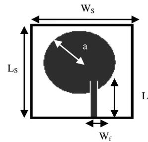
FIG. 1. (A) 0<sup>TH</sup> ITERATION STAGE OF CIRCULAR FRACTAL ANTENNA,
