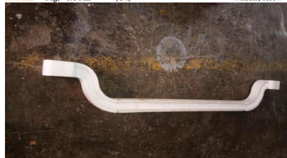
Fig19- Thermocol Pattern CASTING PROCESS
