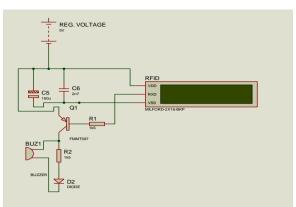
Fig 3: Circuit Diagram of RFID Unit
