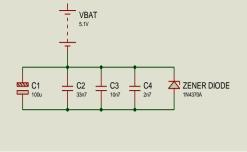
Fig 4: Power Supply to GSM Unit
