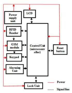
Fig. 1: Block Diagram of the proposed Lock system
