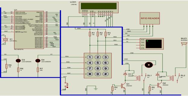
Fig 5: complete circuit diagram of RFID-GSM based lock system
