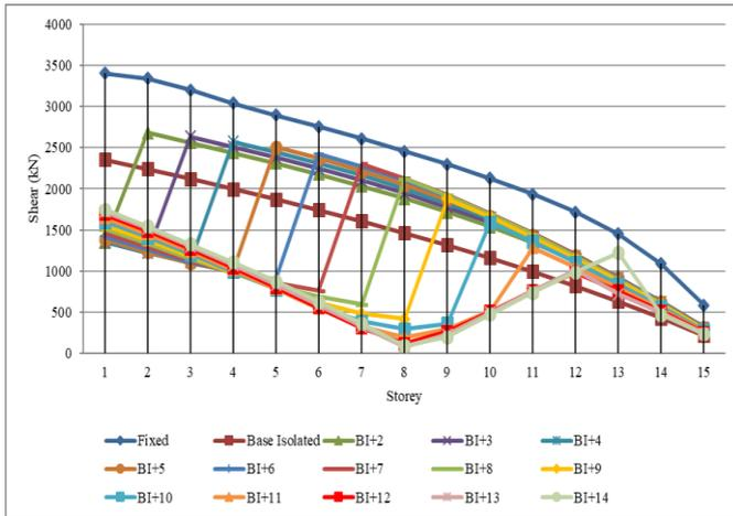
**Fig. 8:** Storey shear for RSX load case.
