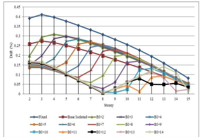
**Fig. 6:** Storey drift for RSX load case.
