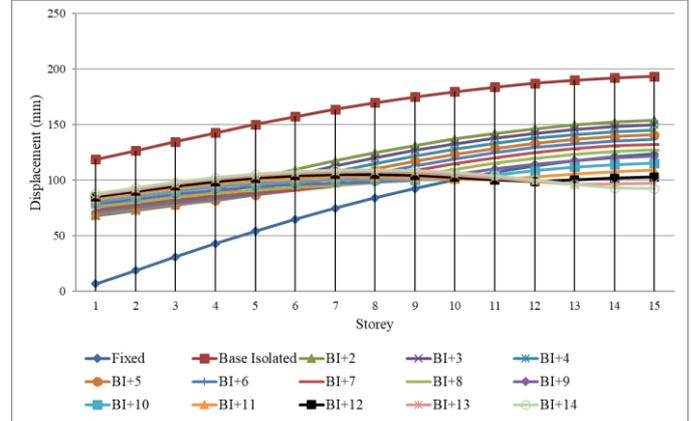
**Fig. 5:** Storey displacement for RSX load case.
