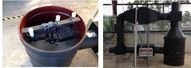
**Figure 1:** Photographs of the parchment coffee dehydration prototype systems. **Left:** open rotary drum dryer referred to as the opened-batea (OB) configuration. **Right:** HARC<sup>2</sup>S referred to as the closed-batea (CB) configuration. The top middle component is the HX that removes dehydration water from the thermodynamic cycle.
