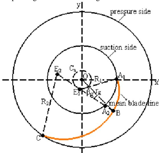
**Figure 6: Representation of the mean blade line using Double Arc Synthetic Method**
