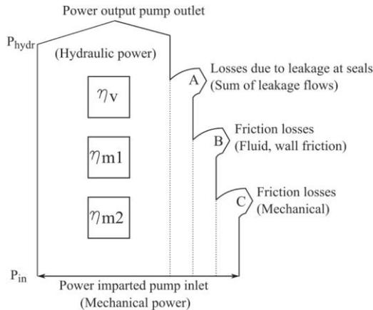
Fig.1 Block diagram showing different losses.
