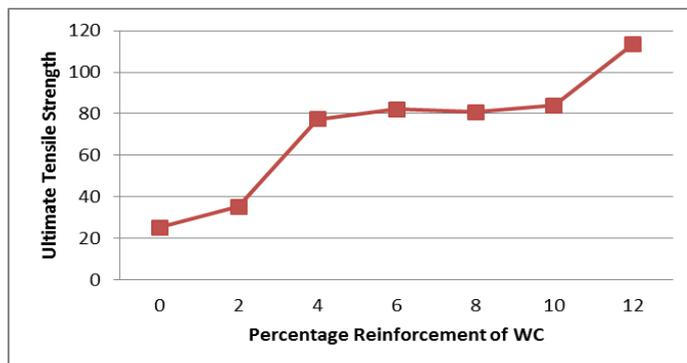
Fig6. Ultimate tensile strength v/s Percentage Reinforcement WC
