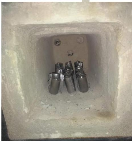
Fig3. Muffle furnace and Sintering of specimens
