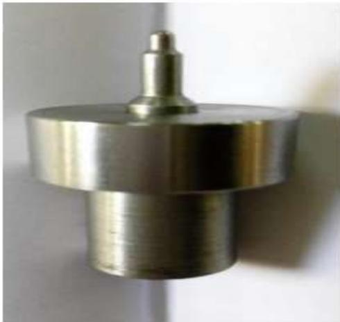
Figure 3.4 Punch in a punch holder
