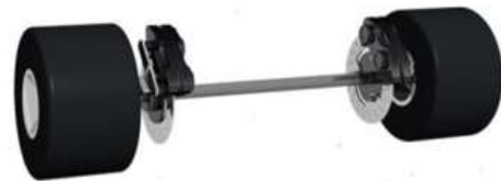
Fig. 13: Disk Brake Arrangement
