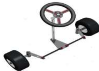
Figure 12: Ackermann steering arrangement
