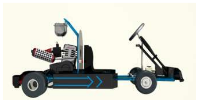
Figure 2: Side View of CAD Model of Go- Kart
