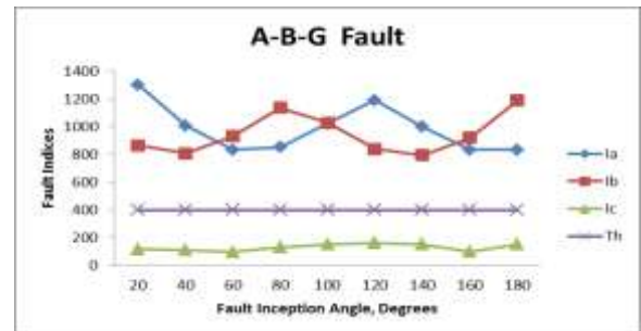
Fig.8 Variation of three phase indices with fault inception angle for A-B-G fault
