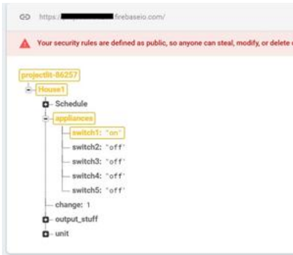
Figure 11: Firebase Console with switch1 ON
