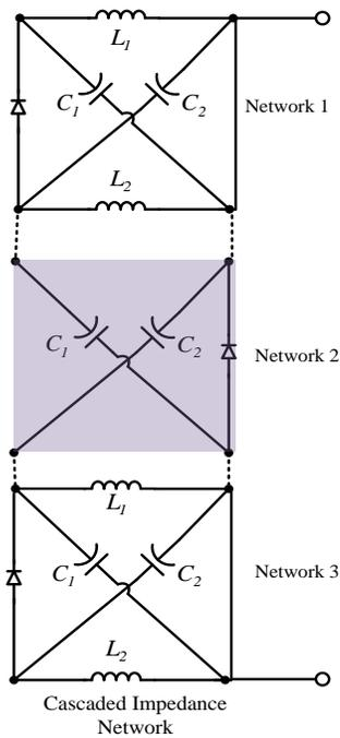
Fig.2. Alternate Cascading
