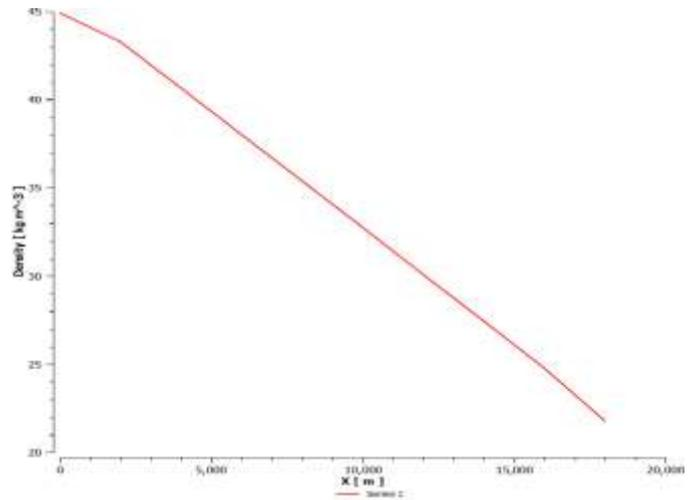
Figure 9: Density distribution along the length of the pipeline with Shell data
