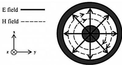
Fig.1. **E** and **H** fields on the coaxial line
