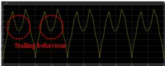
Figure 19: Turbine power versus Time at P max set to 7000
