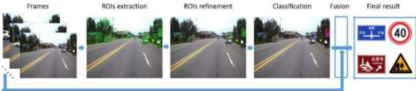
Fig. 2. Pipeline of the proposed traffic sign recognition system
