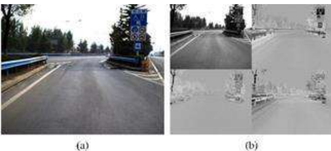
Fig. 3. Raw color image and four channels used to extract MSERs. (a) Original color image. (b) Gray and normalized R,G,B channel.
